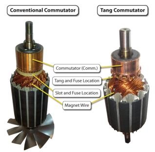
wire and the comm resulting in a relatively inexpensive part cost. However, the connection is not as robust as a conventional comm. However, improved winding methods, better commutator materials, and added secondary operations (such as adding slurry around the tang area and magnet wires) has allowed tang comms to be used in applications that would have been considered too severe in the past.
